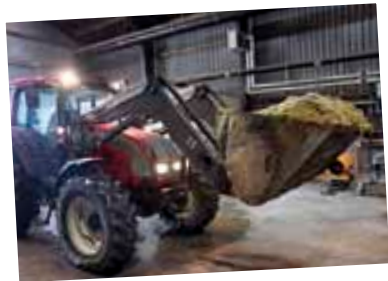
Valtra's biogas tractor was at its best when used for short everyday tasks. When used for loading three hours a day, the tractor had to be tanked every other day.
