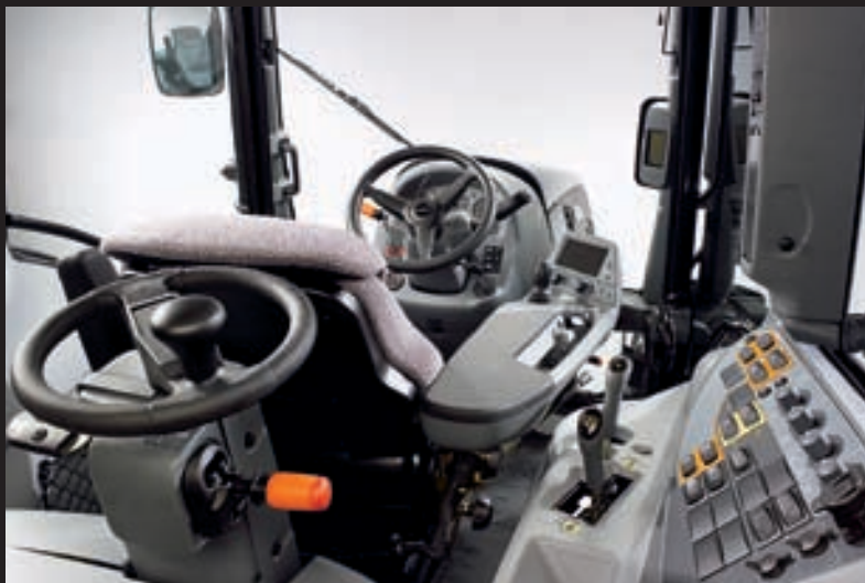
The cabs on the Versu and Direct models are extremely spacious, as there are no gear levers. The rear side window can also be opened
