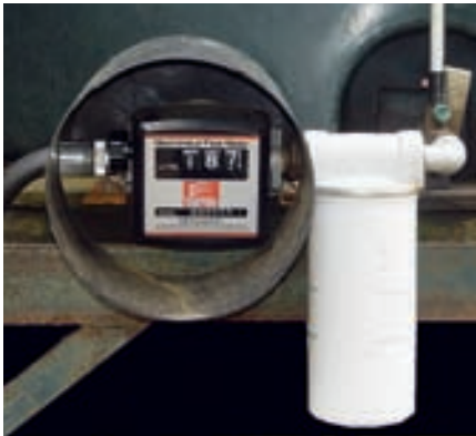
A filter on the tank is Geoff Henwood's starting point for fuel economy.
