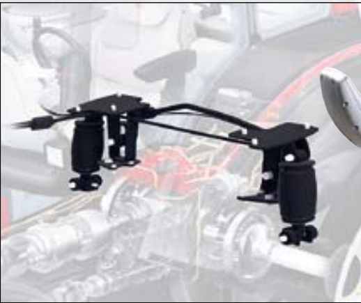
AutoComfort semi-active cab suspension is a unique to Valtra tractors and was awarded at the Agritechnica exhibition with the silver Innovation Award.
