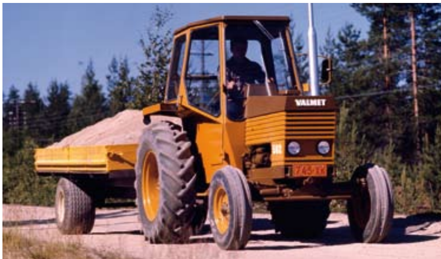
The Valmet 502 stood out from other tractors of the time. The tractor's three-cylinder Valmet 310B engine had a capacity of 2.7 litres and produced 54 hp SAE/2 300 rpm. The partially synchronised transmission featured six forward and two reverse gears. The unloaded weight of the tractor was 2 495 kilos.
