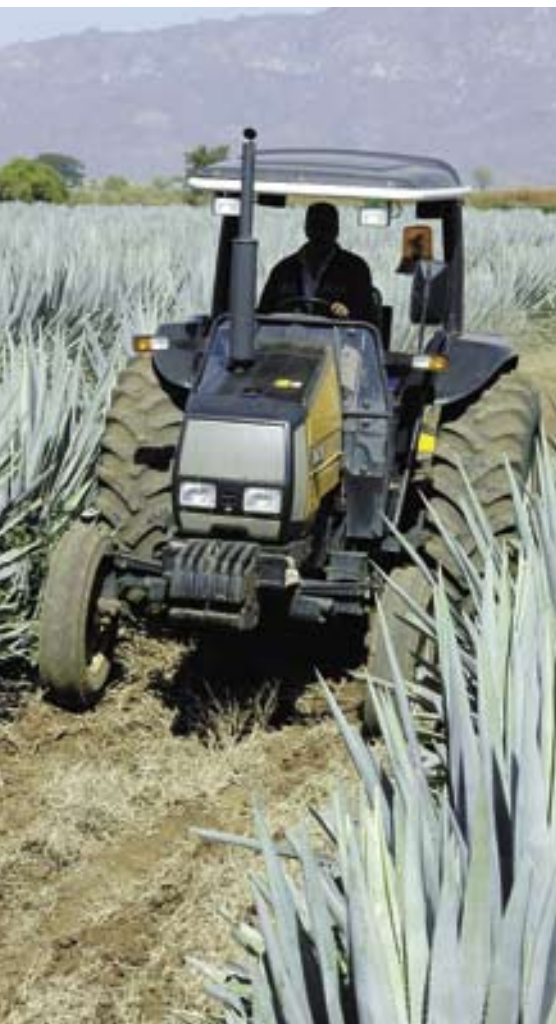
Sausa Tequila has around 100 rear-wheel-drive tractors producing from 50-80 horsepower. These agile, reliable and relatively powerful machines are at home between the rows of agave. The Valtra 700 has been particularly popular, and there are already 40 of them on the Sausa farm.
