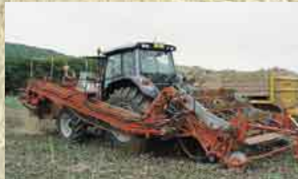
Unusually this machine lifts all four rows in the bed at one pass unlike most other harvesters.
